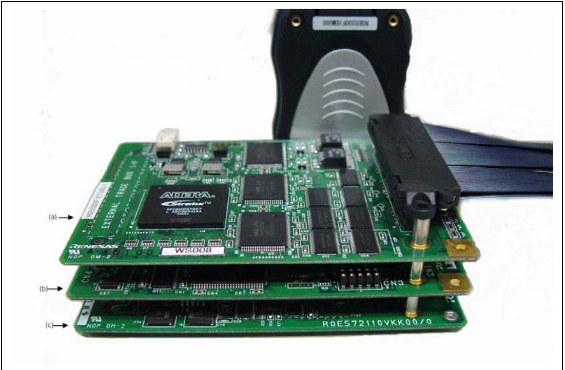
Figure 2.8 Connecting the External Bus Trace Unit, Emulation Memory Unit, and EV-chip Unit
