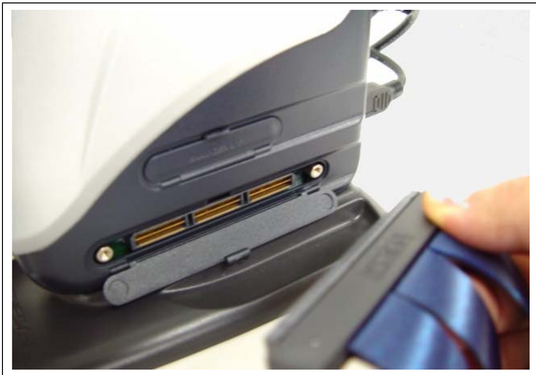
Figure 2.19 Connecting the Trace Cable to E200F
